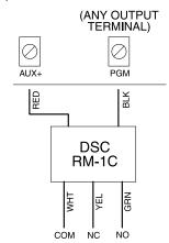
PGM1 can sink up to 50mA of current. Connect the positive side of the LED or buzzer to AUX+, the negative side to PGM1. PGM2 operates similarly to PGM1. However, PGM2 can sink up to 300mA of current. If more than 300mA of current are required, a relay must be used.
